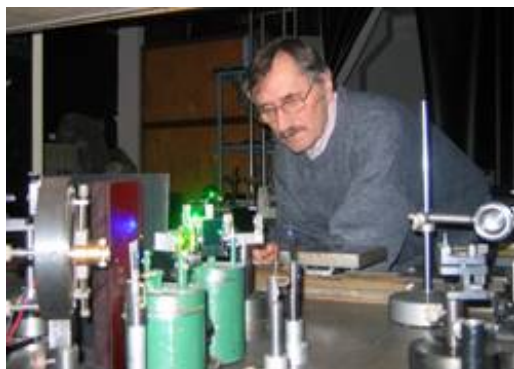
Dr. Jānis Teteris preparing holographic recording in thin semiconductor films
