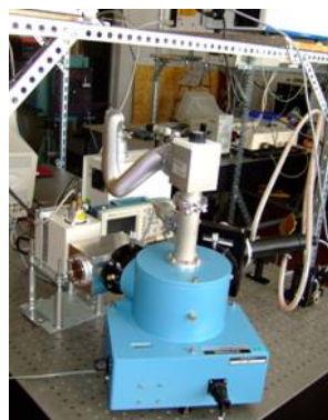
Spectrometer for studies of optical properties of materials in vacuum ultraviolet range
