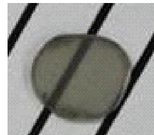
Fig 1. Sintered sample of Ce/Al/Mg:SrHfO 3 ceramics pre-sintered at 1,400°C. Diameter is 10 mm.
